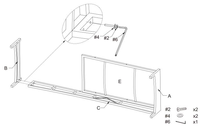
Step 4. Attach left side panel (part D) to front panel (part A), back panel (part B) and seat panel (part E) using bolts (part #2), washers (part #4) and allen key (part #6).
