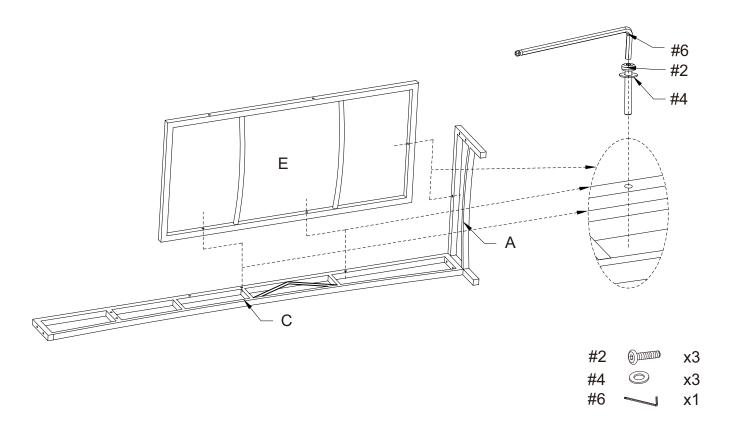
Step 3. Attach back panel (part B) to right side panel (part C) using bolts (part #2), washers (part #4) and allen key (part #6).
