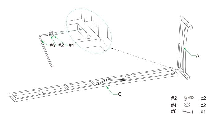
Step 2. Attach seat panel (part E) to right side panel (part C) and front panel (part A) using bolts (part #2), washers (part #4) and allen key (part #6).
