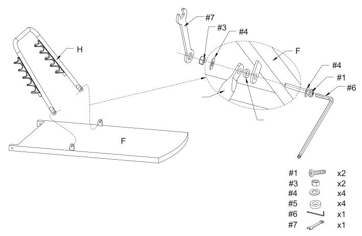
Step 7. Attach the assembled unit (parts F&H) to right side panel (part C) and left side panel(part D) using bolts (part #2),washers (part #4) plastic washers (part #5)and allen key (part #6).
